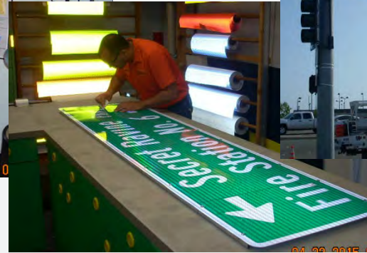
Apply material to aluminum sign backing
